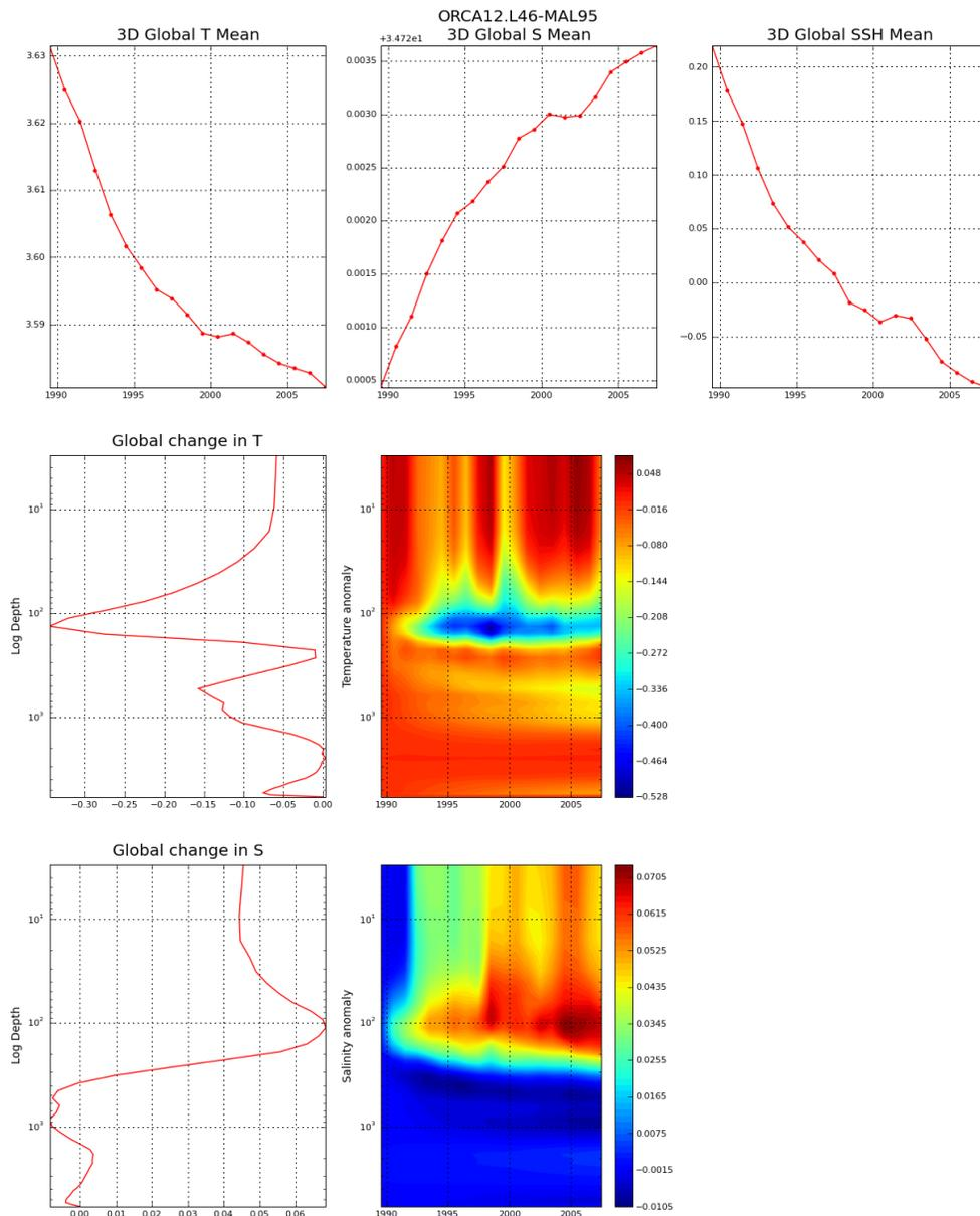
Figure 9: Top plots: Year-to-year variations of the world ocean average temperature and salinity over the integration period (1989-2007). Middle and bottom plots: Changes compared to initial condition in horizontally averaged temperature and salinity (vertical logarithmic depth range), left is the final minus initial profile, and right is the time evolution of the difference with initial condition.
